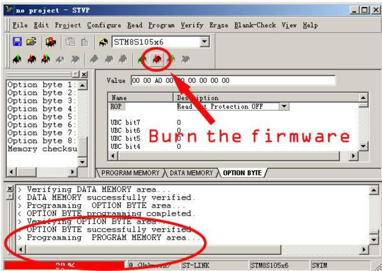
If all fine, after burn the firmware, unplug the wires and re-power the clock to see the result.
