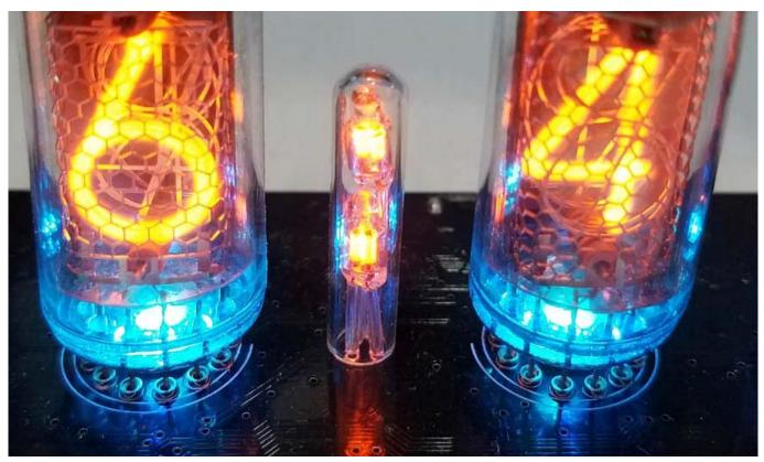
And if you feel necessary, after plug the middle legs into the sockets, you can use sharp scissors to cut the bulbs' legs short on the back side of the PCB. And in order to prevent some guys pull the middle dots out the sockets when the clock in working, you can band the middle bulbs legs into 90 degree or even into a fish hook looking (do not short the legs). And the last thing about the middle dots is please do not twist the middle dots or will short the circuit.
